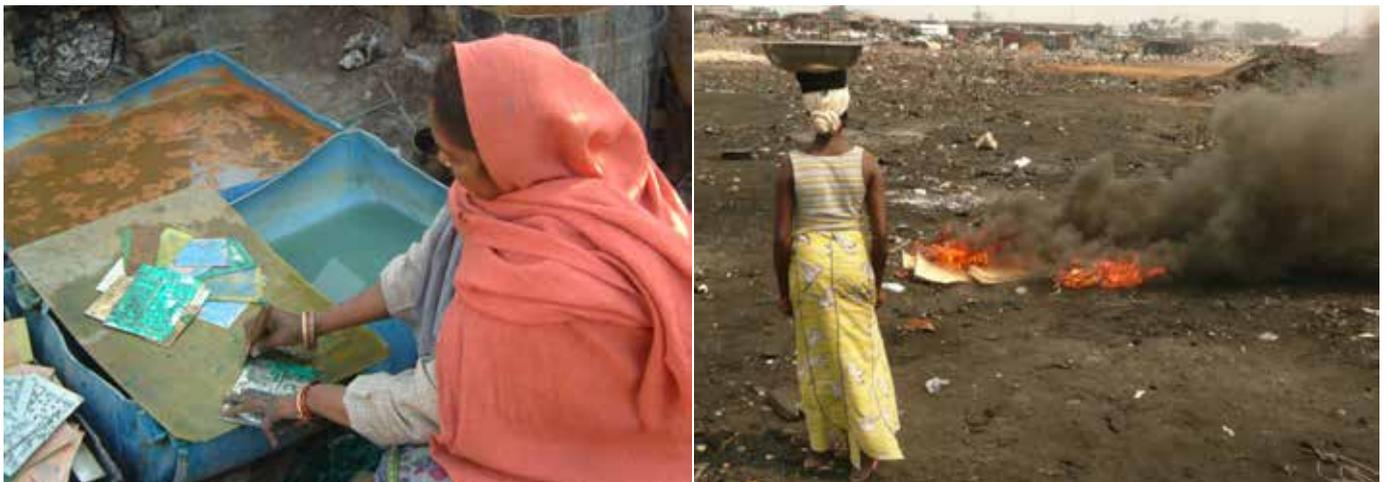
**Figure 3:** The informal sector in developing countries often uses inappropriate recycling techniques such as acid leaching of gold (left, India) and burning of cables to recover copper (right, Ghana)
