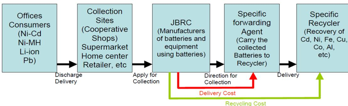
**Figure 6:** Process of collecting and recycling of compact rechargeable batteries in Japan (Source: Kunitomo 2006 [10])
