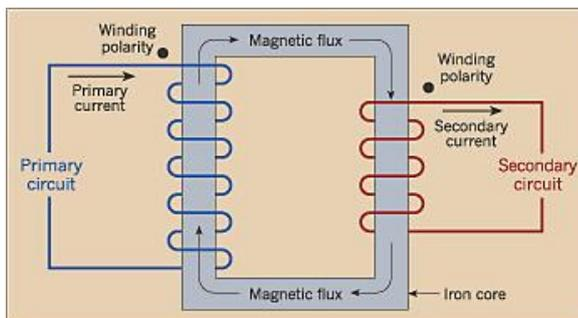
Graph 6: Principle of an electric transformer
