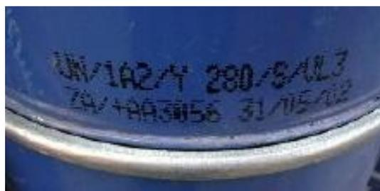
This container must be clearly marked with a specific label for the transport of hazardous chemicals with details of the contents and must be maintained in good condition. **Graph 15: Imprinted UN Code of an UN approved drum**
