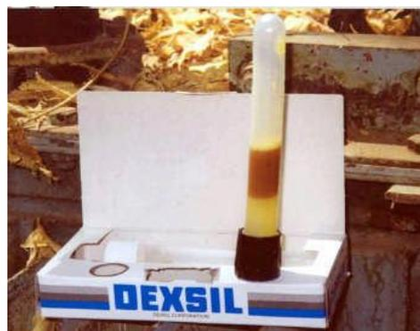
Graph 11: PCB screening with a test kit
