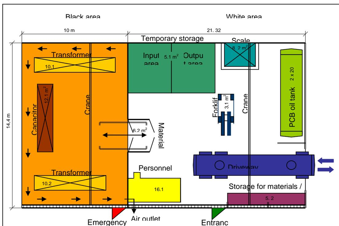
**Graph 14: Sketch of a temporary storage site for PCB contaminated electrical equipment (transformers, capacitors)**
