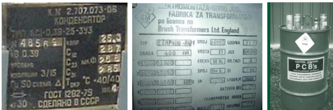
**Graph 9: Identification plates and labels for identifying electrical equipment and containers with PCBs**
