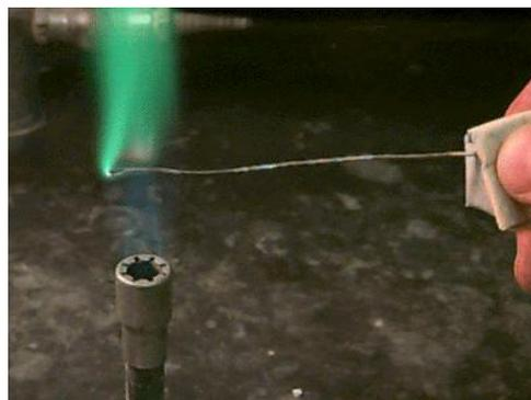
Graph 10: Beilstein's test for chlorine
